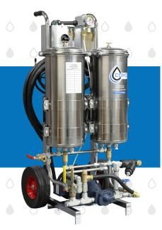
The COMO Model 120 specializes in the efficient removal of excess water from your oil-based fluids. First, a pre-filter removes the largest contaminants. Next, the coalescing filter separates the water from the oil. Finally, the COMO depth filter polishes the oil, removing water to as low as 20 ppm, and particles down to 1  $\mu$ m.
