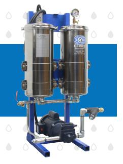
The Model 265 is designed for kidney-loop filtration of a single machine. With dozens of filter options, you can meet your exact cleanliness goals—as low as 1  $\mu$ m and 20 ppm water. Each COMO Filter holds up to 20 pounds of dirt and 1 gallon of water, so you can extend fluid life and reduce downtime with fewer filter changes than the competition.
