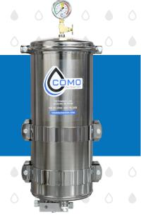
COMO's Safety Valve Filter Housings allow you to install a COMO bypass depth filter directly to a high pressure hydraulic system without exceeding the filter vessel pressure rating. Our safety valves will maintain a maximum 60 PSI within the housing while allowing constant flow for continuous contamination control.
