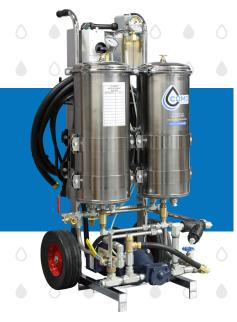
The Model 130 specializes in applications with large contaminants. A filter-bag removes large particles before the COMO Filter polishes the fluid to any cleanliness level you desire. Each COMO Filter holds up to 20 pounds of dirt and 1 gallon of water, so you can extend fluid life and improve machine performance with fewer filter changes.
