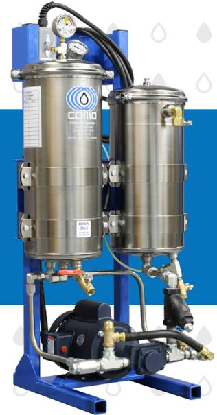
The Model 165-400 excels in applications with large contaminants. A filter-bag removes large particles before the COMO Filter polishes the fluid to any cleanliness level you desire. Each COMO Filter holds up to 20 pounds of dirt and 1 gallon of water, so you can extend fluid life and improve machine performance with fewer filter changes.
